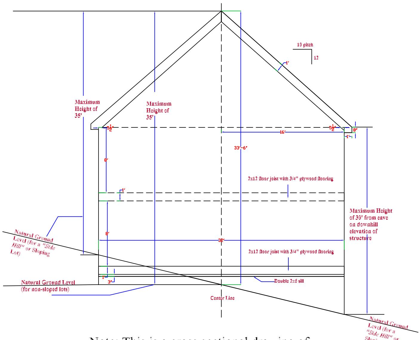
Note: This is a cross sectional drawing of a standard New England Colonial style home with a base width of 32'. Each floor has a thickness of 12" and a wall height of 8'. The roof has a 10 pitch for a total height from the "Natural Ground" to the ridge of 33'-6".
